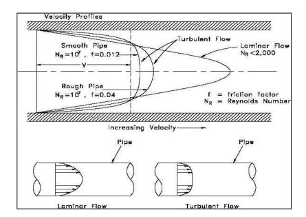
Figure 2 : Laminar and turbulent flow velocity profile
