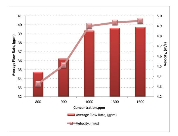
Figure 6: Graph for Average Flow Rate (gpm) and calculated Flow Velocity (m/s)
