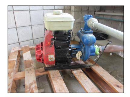
Figure 15: Engine pump
