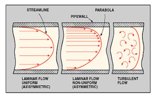
Figure 1: Laminar flow and turbulence flow in a pipeline side view
