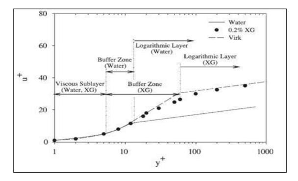
Figure 3: Thickness of buffer layer in water and Xanthan solution (polymer), (Escudier, M.P., & Smith, 1999)
