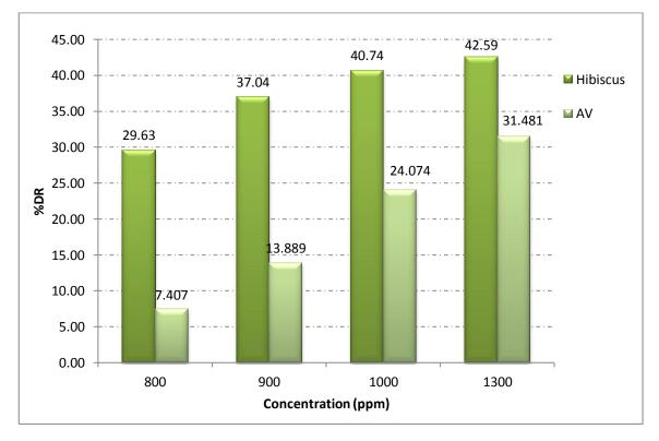
Figure 11: Comparison of drag reduction vs. concentration
